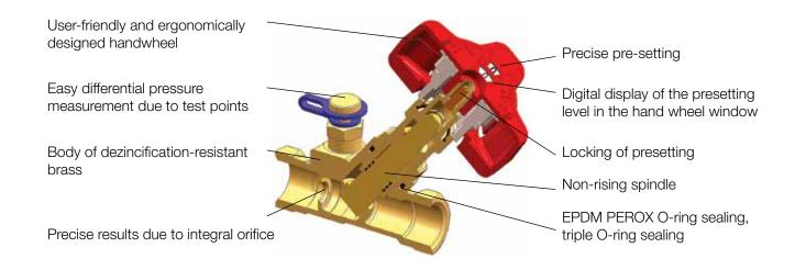
4017 M and 4017 ML: 2 test points for differential pressure measurement at the integral orifice; test points in extended version available as accessories.
